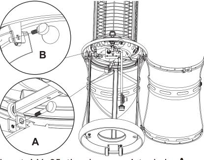
Insert M6x35 thumb screw into hole  $\bf A$ , and M6x12thumb screw into hole  $\bf B$ . Lock the screws.
