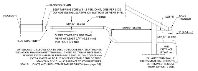
NOTE: MAKE SURE THAT ALL FLUE/EXHAUST JOINTS ARE SEALED. USE ONLY SUITABLE PRODUCTS EQUAL TO GENERAL ELECTRIC RTU 106 OR PERMATEX FORM A GASKET RED HIGH TEMPERATURE SILICONE ADHESIVE SEALANT. (NOT SUPPLIED)
