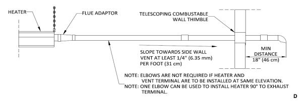
NOTE: VENT PIPE CAN BE TRIMMED IF NEEDED. CUT EXCESS MATERIAL AS REQUIRED. MAINTAIN 6" (16 cm) CLEARANCE TO COMBUSTIBLES. SEAL ALL JOINTS WITH HIGH TEMPERATURE SILICON (SEE PAGE Error! Bookmark not defined.).
