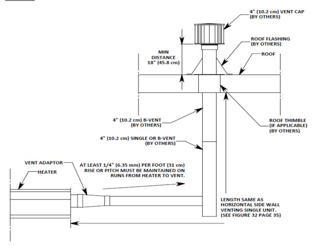
Figure 16. VERTICAL VENTING, SINGLE UNIT
