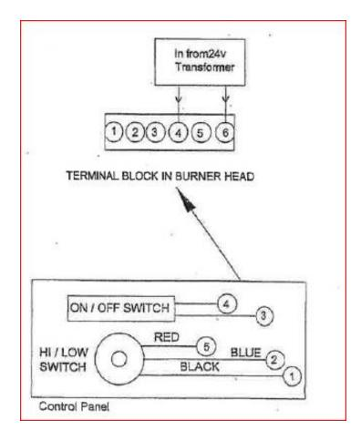
Figure 22. ELECTRICAL CONNECTIONS 24 VOLT
