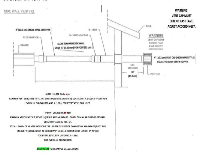
NOTE: MAKE SURE THAT ALL FLUE/EXHAUST JOINTS (AND SEAMS IF NECESSARY) INSIDE AN OCCUPIED BUILDING ARE SEALED. USE ONLY SUITABLE PRODUCTS EQUAL TO GENERAL ELECTRIC RTU 106 OR PERMATEX FORM A GASKET RED HIGH TEMPERATURE SILICONE ADHESIVE SEALANT. (NOT SUPPLIED)
