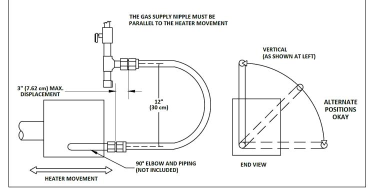
Figure 19. GAS LINE CONNECTION WITH CERTIFIED FLEXIBLE GAS CONNECTION
