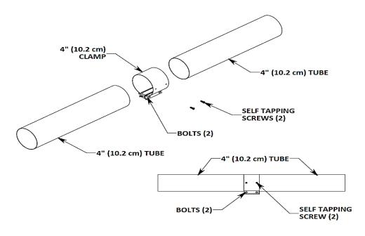
Figure 11. CLAMP COUPLER INSTALLATION
