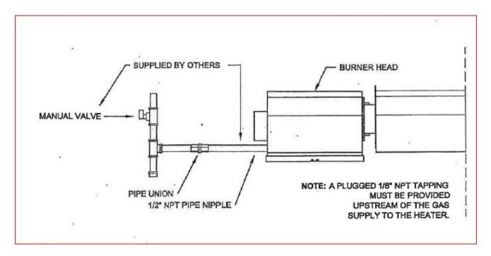
Figure 18. HARD PIPE INSTALLATION
