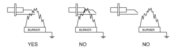
Figure 24. PROPER ELECTRODE LOCATION
