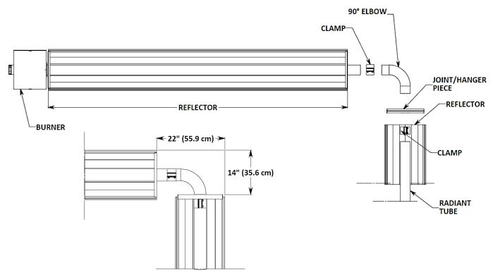
Figure 13. 90° ELBOW KIT INSTALLATION
