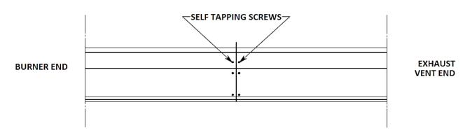
Figure 10. JOINT HANGER INSTALLATION
