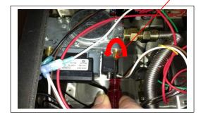
6) Connect a manometer that registers pressure in inches of water column ("W.C.) to the manifold pressure tap.
