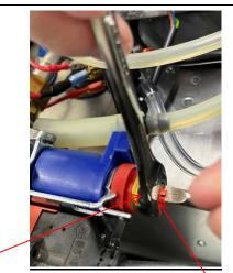
12) If adjustment is needed, hold the high pressure adjustment nut in place with a 10mm wrench. Use a small slotted screwdriver to adjust the low pressure adjustment screw (bright orange plastic head). Turn counterclockwise to lower pressure and clockwise to increase pressure.
