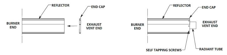
Figure 12. END CAP INSTALLATION
