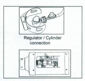
If NO bubbles appear at any connection, the connections are secure.
