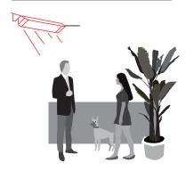
Angle fixture 30° to 60° from horizontal face down. Best angle is approximately 45°.
