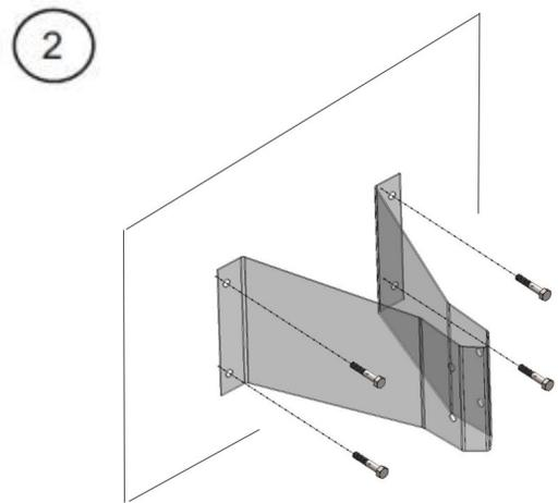
FASTEN WALL BRACKET TO STRUCTURE USING FIELD SUPPLIED FASTENING HARDWARE. ENSURE SUFFICIENT STRENGTH AND INTEGRITY TO CARRY WEIGHT OF HEATER AND WIND/ SNOW LOADS
