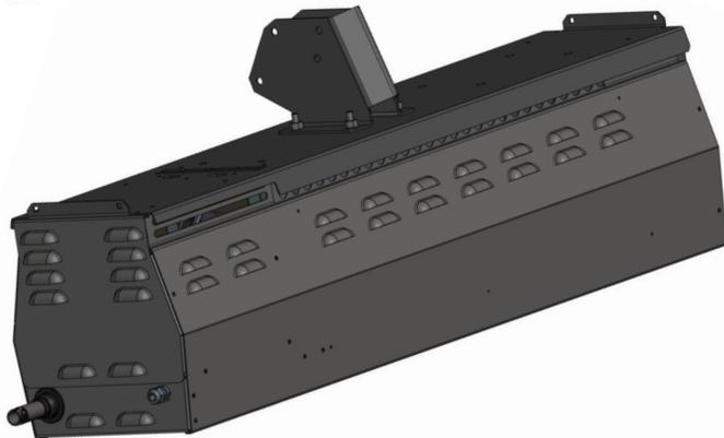
4 INSTALL HEATER BRACKET ON TO WALL BRACKET USING BOLTS SUPPLIED [INSERT TOP BOLT FIRST TO CARRY WEIGHT OF HEATER]
