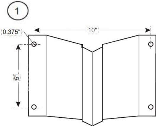
USE BRACKET AS TEMPLATE FOR HOLES/BOLTS TO THE STRUCTURE. FASTEN TO STRUCTURAL MEMBER[S] OR DEVISE STRUCTURAL SUPPORT TO CARRY WEIGHT OF HEATER AND WIND/ SNOW LOADS
